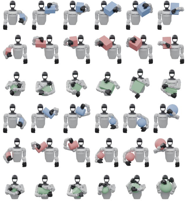
Fig. 6: Example whole-body grasp configurations. Authored torso-and-arm postures and object transforms are restored together at reset. These illustrate initialization geometry, not cross-object policy evaluation.
